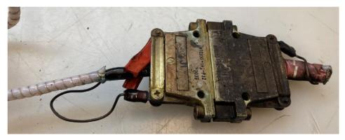
Figure 28. Left pull down actuator showing the electrical grommet of the connector.
