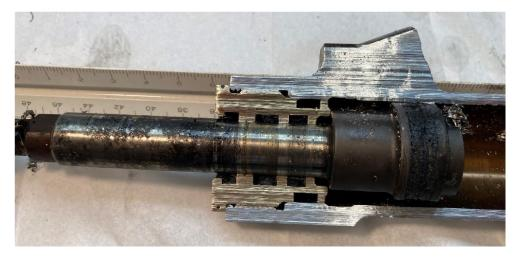
Figure 4. Right lift dump actuator after sectioning – half 1.
