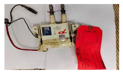
Figure 37. Right Aileron Trim Actuator.
