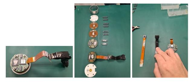
Figure 1: (Left). View of memory puck with base cover removed, showing the memory PCB. (Centre): Each layer of the memory puck is removed. (Right): Verification of the replacement cable to be used.
