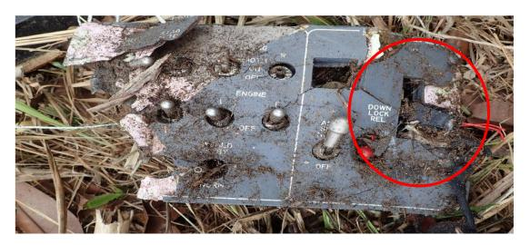
Figure 10. Landing Gear Handle.
