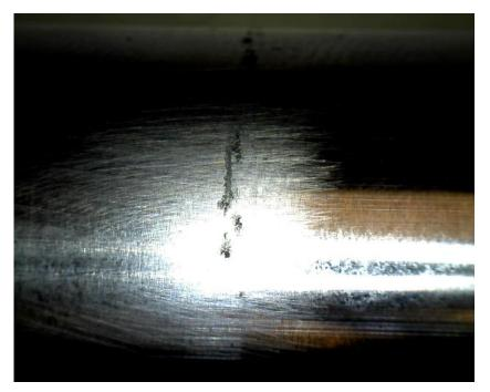
Figure 26. Left roll control actuator piston showing the abrasion area under a microscope.
