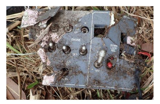
Figure 9. Damaged Landing Gear Handle.
