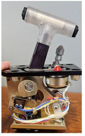
Figure 3. Exemplar lift dump handle – showing the right side in the RET (retract) position. (Courtesy of Textron Aviation).
