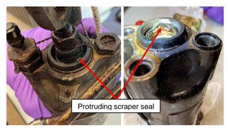
Figure 31. Left pull down actuator showing the protruding scraper seal on the rod end of the actuator.
