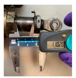
Figure 8. Right roll control actuator as received extension dimension.
