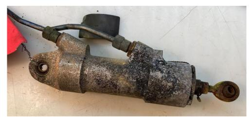
Figure 16. Left lift dump actuator.
