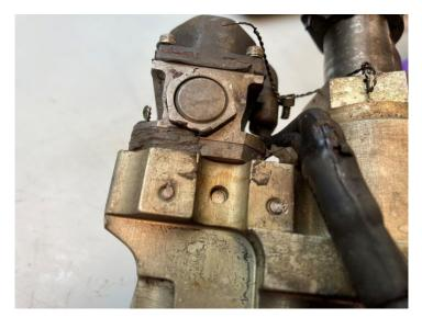
Figure 7. Right roll control actuator showing where the cable retainer screws for the wire harness retainer were sheared off.
