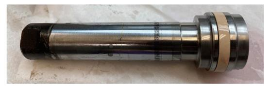
Figure 24. Left roll control actuator piston showing the seal material transfer area.
