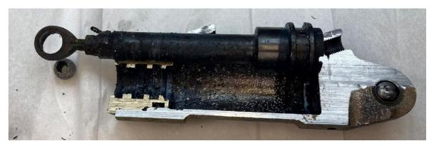
Figure 19. Left lift dump actuator after sectioning – half 1.
