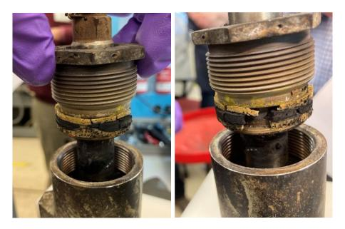
Figure 3. Right lift dump actuator gland nut after removal.
