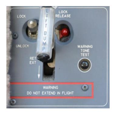
Figure 16. Photograph of an Exemplar Lift Dump Panel
