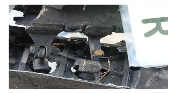
Figure 16. Right lift dump panel down-lock striker and locking actuator.
