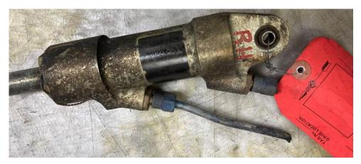
Figure 1. Right lift dump actuator.
