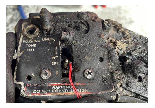
Figure 10. Lift Dump Handle Found in Intermediate Position.
