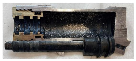
Figure 20. Left lift dump actuator after sectioning – half 2.
