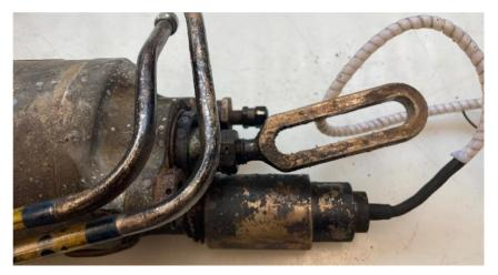
Figure 30. Left pull down actuator showing the bent slotted rod end.
