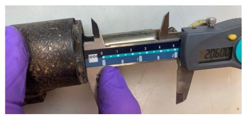
Figure 2. Right lift dump actuator extension dimension.
