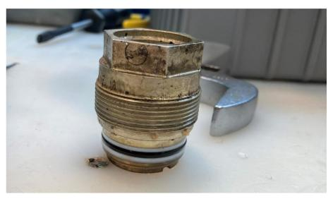
Figure 9. Right roll control actuator gland nut after removal.
