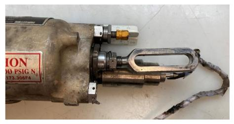
Figure 12. Right pull down actuator showing the bent slotted rod end.
