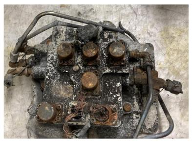
Figure 35. Spoiler Hydraulic Control Module.
