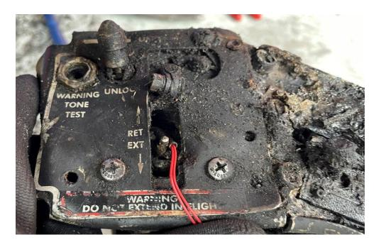
Figure 15. Lift Dump Panel
