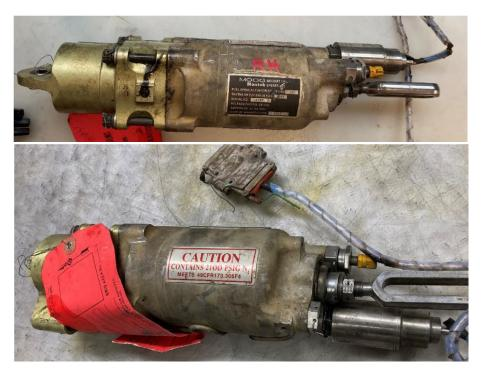
Figure 11. Right pull down actuator.
