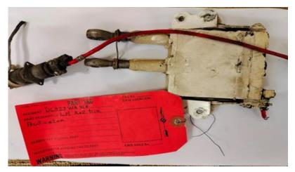
Figure 38. Left Aileron Trim Actuator.
