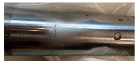
Figure 25. Left roll control actuator piston showing the abrasion area and material deposits.
