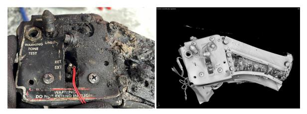
Figure 11. Lift Dump Panel (Left) and CT Image of the Panel (Right).
