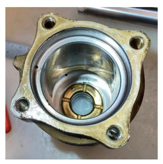
Figure 14. Right pull down actuator showing the inside of the cylinder.
