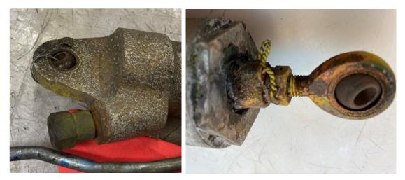
Figure 17. Left lift dump actuator tail side and rod end bearings.
