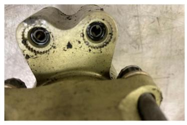
Figure 13. Right pull down actuator showing hydraulic ports.
