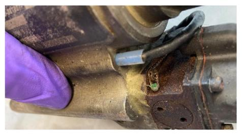
Figure 22. Left roll control actuator showing sheared safety wire near the servo valve.
