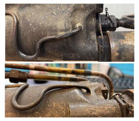
Figure 29. Left pull down actuator showing the crushed transfer tube.
