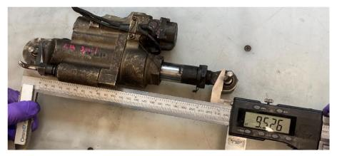
Figure 23. Left roll control actuator as received inside pin to pin measurement (must add 0.31 pin diameter to get actual pin to pin measurement).
