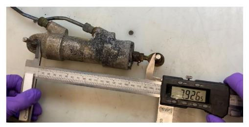
Figure 18. Left lift dump actuator inside pin to pin measurement (must add 0.31 pin diameter to get actual pin to pin measurement).
