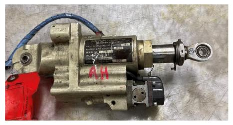
Figure 6. Right roll control actuator.
