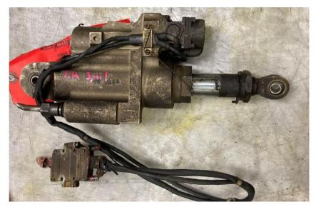
Figure 21. Left roll control actuator.
